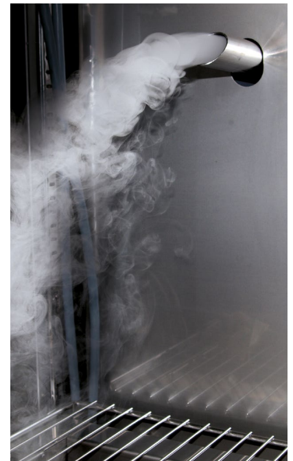
Aerosol mist without heat introduction into the test room.
