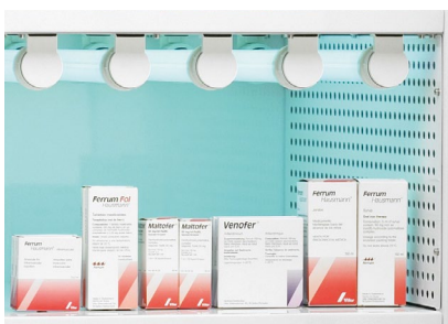
Photo stability tests of drugs according to ICH Q1B.
