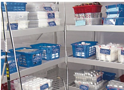
Stability test of drugs according to the ICH Guideline in the climatic chamber.
