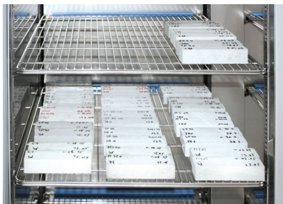
Freeze-thaw alternating tests in building material testing show the durability of the material.
